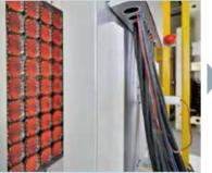
Asano Laboratories Co., Ltd. Ouick Response Heater 6kW×81Heaters×2set (Upper and Lower) (48.6kW/m2) Material Hand Robot Available for Any kind of Material
