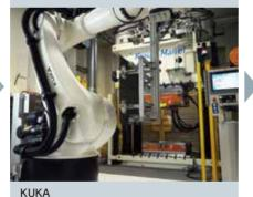
Material Hand Robot KR 240 R3330 Loading Capacity: 240kg
